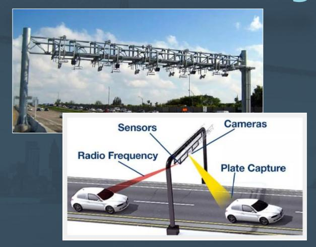
Gantries with sensors and cameras will scan the ALGO pass or capture a picture of the license plate. No slowing or stopping.
