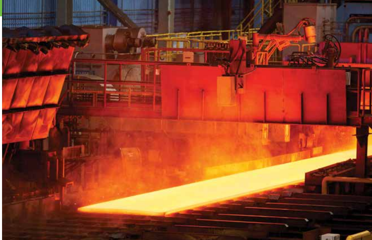
A heated steel slab before it is rolled at AM/NS.
