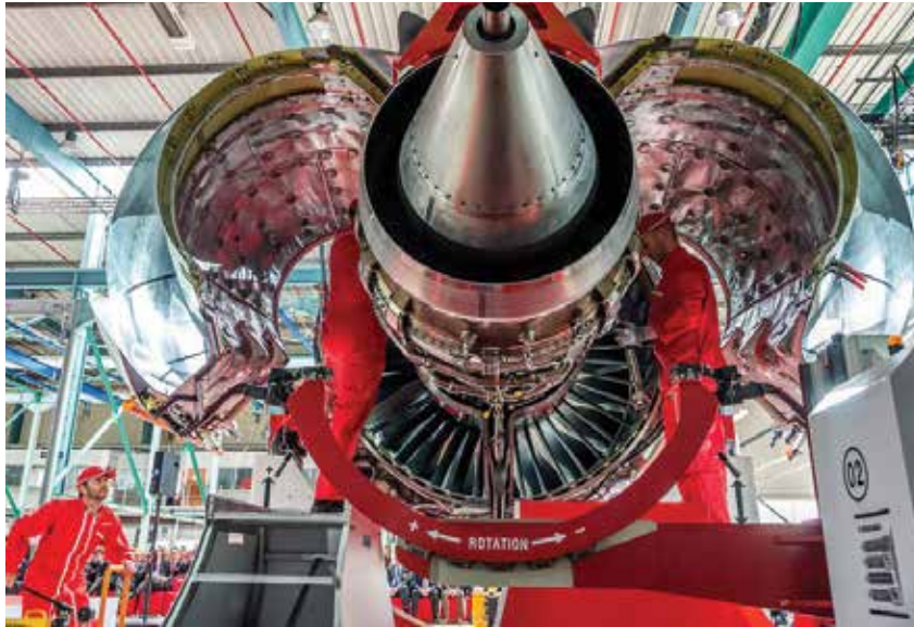
Above is an integrated propulsion system with a nacelle, similar to what will be made in Mobile once Safran USA begins operation.
